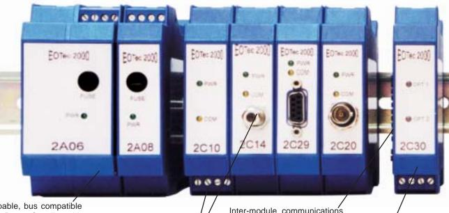
Hot-Swappable, bus compatible Redundant Power Supplies with diagnostic outputs to eliminate single point of failure, reducing the risk of significant costly system down-time
