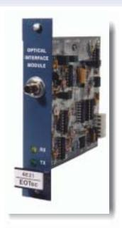
The exclusive 6E21 Ping-Pong optical module provides bi-directional communications on a single fiber cable.
