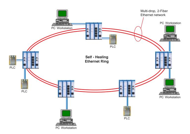
This diagram shows a typical Ethernet ring configuration using the fiber optic Media Converters/Hub assembly. This topology enables a self-healing network functionality.
